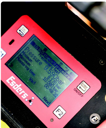
Mobile pressure meter device which is used for successively testing all network connections.
